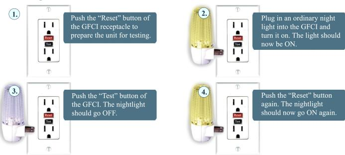
The nightlight should turn off when the "TEST" button is pushed. If the light does not turn off, then the GFCI could have been improperly wired or damaged and may not offer shock protection. Contact a licensed electrician to check the GFCI and correct the problem.
